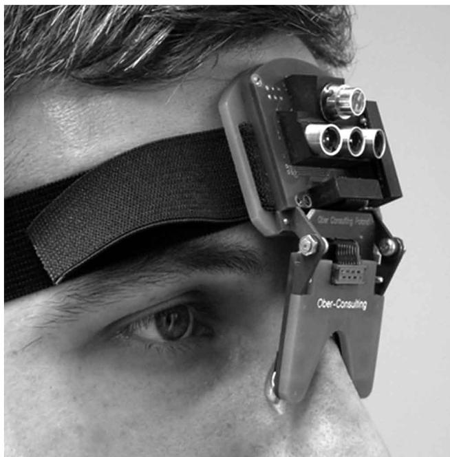
Fig. 1. Saccadometer Advanced, the forehead plate carries the laser stimulator assembly (one green and three red) and provides the conditions for effective cancelation of vestibulo-ocular responses, improving the stability of eye fixation on the displayed targets, necessary for high temporal resolution detection of saccades onset and landing
