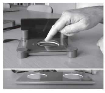
Fig. 4. Tapping Pad, at the bottom the low profile sensor plate, provides the possibility to rest the forearm on the table. At the top – the tapping pad with an attached transparent overlay with the vertically oriented obstacle, separating two sensor surfaces. The obstacle not only physically extends the path of the lateral hand movements, but also make it more complex to control (involving vertical component).
