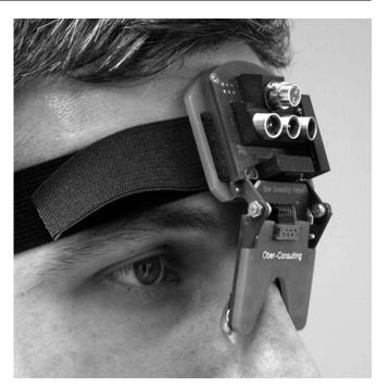
Fig. 1. Saccadometer Advanced, the forehead plate caries the laser stimulator assembly (one green and three red) and provides the conditions for effective cancelation of vestibulo-ocular responses, improving the stability of eye fixation on the displayed targets, necessary for high temporal resolution detection of saccades onset and landing
